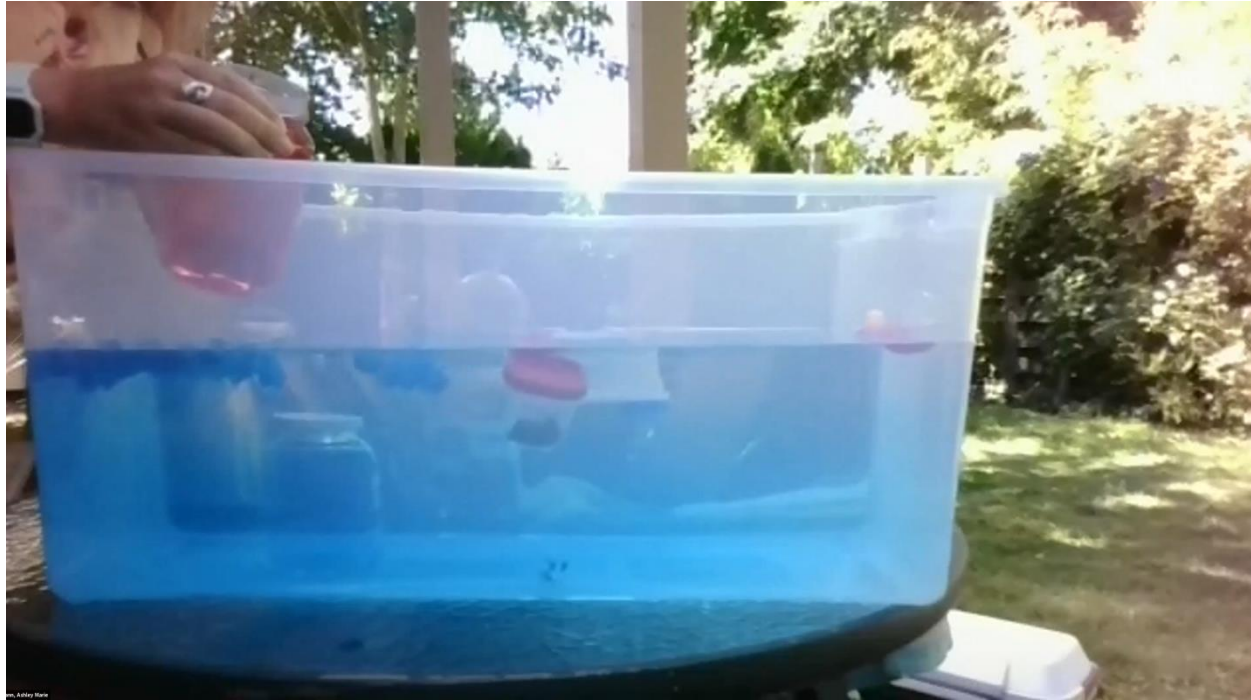
Image 5: Screenshot of the group experiment conducted virtually. Campers discussed how the variables they hypothesized would effect ocean currents were simulated in the experiment materials before testing them. In this example, blue water represents cold water, red water represents warm water, and objects of varying densities are in the tank to test where the “currents” push them.
