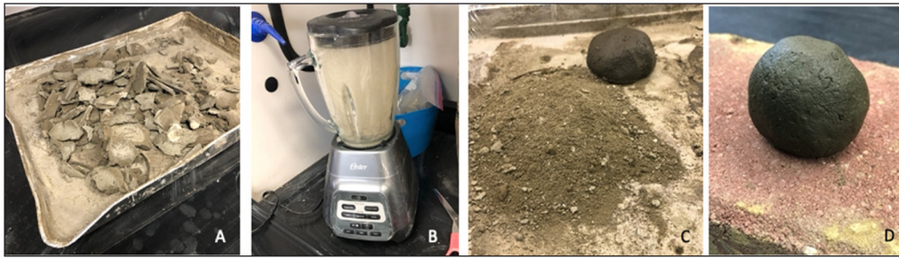
Figure 4 Algal biomass scraped from the surface of a concrete boat-ramp was dried and then broken into smaller fragments (Figure A), ground in a blender (Figure B), turned into a fine powder (Figure C) and then rehydrated to form a moldable clay (Figure D).
